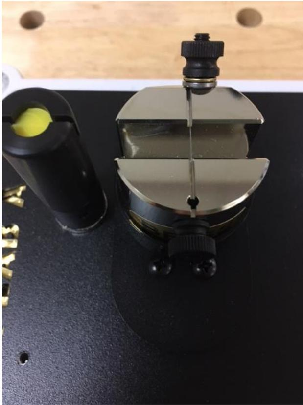
Edge sharpness readings may be taken in much the same way as they are with our PT50 Series units and utilize the same ATF-10G fixture and test media. Press the *MAX* mode key on the instrument keypad. Place the test media fixture on the weigh plate and magnetic base **KF-10L** (elongated version of the KF-10R) knife fulcrum on the Edge Lab cover plate as indicated in the photo below. The instructions that follow are adapted from the PT50 Series **Quick Start Guide**.
