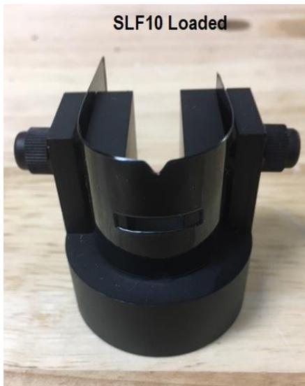
5. Click "Begin Test" and then place knife edge in the "v" shaped notch and then slowly draw/pull knife handle toward the user (keypad) while applying downward force to the blade. Make certain that the blade is held vertical throughout the process and that the slice is straight.
