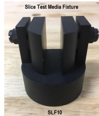
SL100 Test Media is packaged in bundles of 50 and can be used to conduct 100 tests. After completing one test, flip the strip over and conduct the next test. SL100 test media is designed to be used in conjunction with the SLF10 Test Media Fixture.
